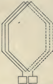
FIG. 176.—Multiple-circuit Winding —three-turn coil.
